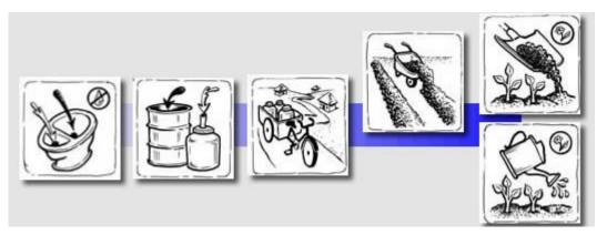
Example of a sanitation chain with a diversion toilet, separate storage for excreta and urine, transport of tanks, composting and re-use of manure and urine (source: www.akvo.org).
